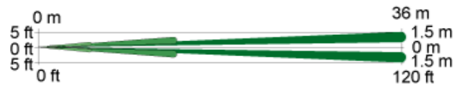
Top View Optional Long Range Coverage: 25 m to 36 m x 3 m (80 ft to 120 ft x 10 ft)
